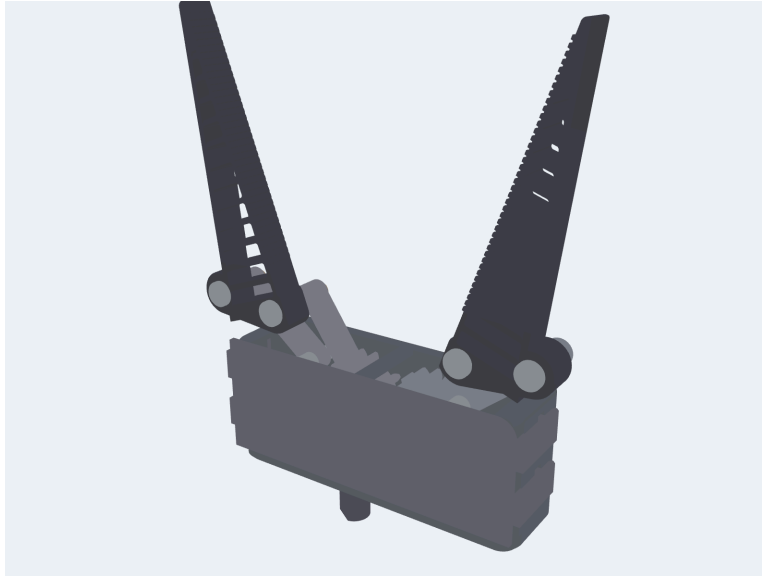
Figure 4.1 The SoftSense end effector in the fully open pose, the two Fin Ray fingers splayed into a funnel-mouth catch.
